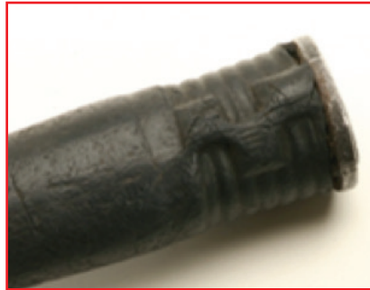
Hose Without A Fitting Shows A Potential Leak Path That Often Allows For Steam Loss When Using Traditional Clamped Fittings
